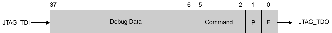
Figure 25-2 Serial Debug Port Data Register Format
