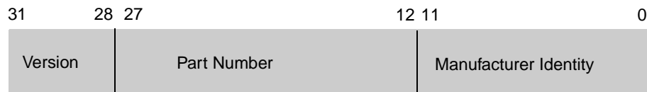
Figure 25-3 Device Identification Register Format
