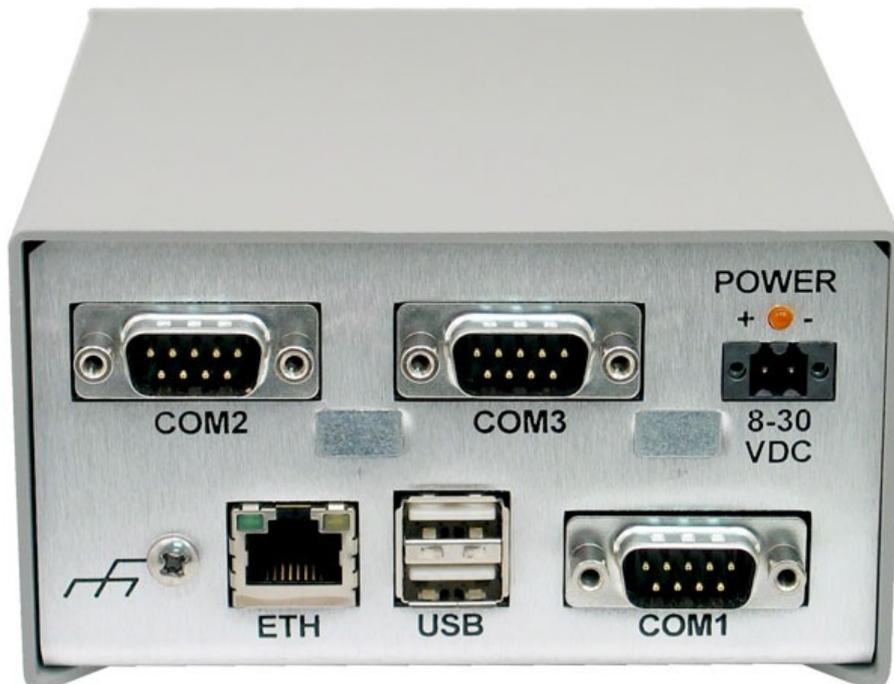
The rear panel of the TS-ENC720 enclosure (shown above) has all of the input/output connectors, including one COM port, two DB9 ports which can be used for an additional COM port, 8 channel A/D, or 8 DIO pins, one ethernet port, two USB ports, two pin power connector, as well as a power indicator LED.
