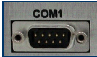
Enclosure TS-530 COM1 Port
