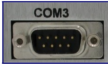
Enclosure TS-540 COM3 Port
